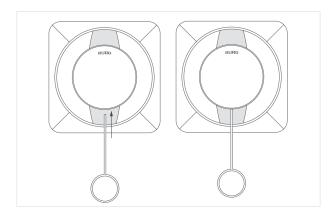
Hold the opening pin in position and turn the pin with the housing (shown as a gray area in the sketch) counterclockwise by approx. 10°. The operating panel is <u>not</u> rotated during this process.
