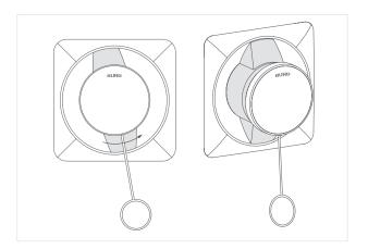
4 Remove the opening pin and pull the operating panel forwards.
