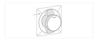
2 Carefully insert the opening pin into the closure hole underneath the operating panel until resistance is reached and press lightly.
