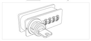
4. Hold the knob. Turn the master key counterclockwise until it can no longer be moved. **Hold the knob and master key in this position.**
