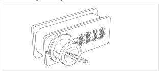
5. Start with the number wheel next to the knob. Carefully turn the number wheel once fully (e.g. from 0 to 0). Repeat the process for the other number wheels.
